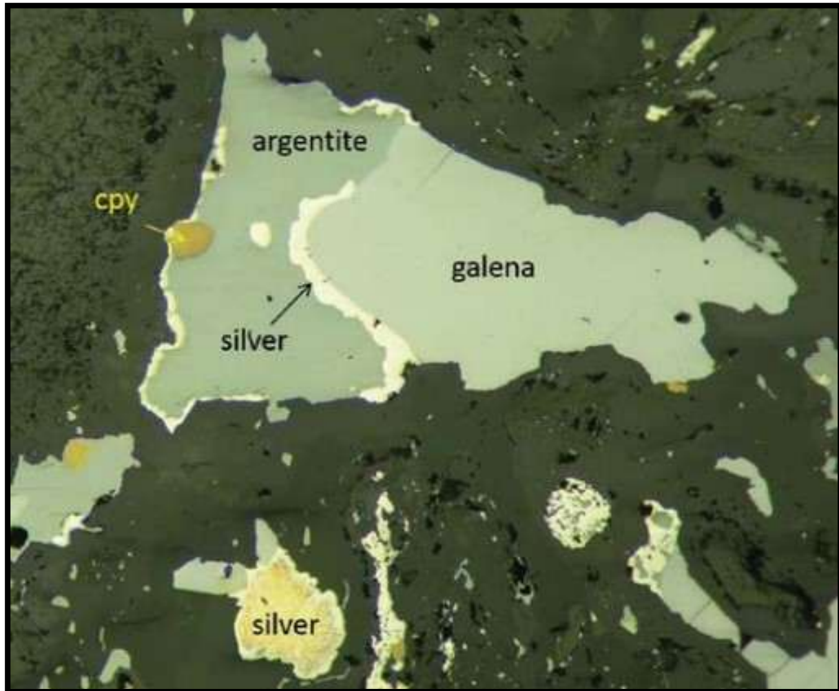
Figure 7-7 A Reflected light Microscopy image of mineralization from the Lexington mine. Visible are native silver, galena (PbS), argentite (Ag 2 S) and chalcopyrite "cpy" (CuFeS 2 ) (Gammons et al, 2016).
