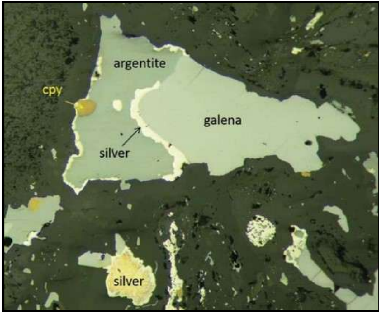
Figure 15: A Reflected light Microscopy image of mineralization from the Lexington mine. Visible are native silver, galena (PbS), argentite (Ag 2 S) and chalcopyrite "cpy" (CuFeS 2 ) (Gammons et al, 2016).
